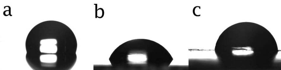
Figure 5. Water contact angles of (a) BIIR, (b) PMMA, and (c) BIIR-g-PMMA after 8 h of graft reaction. Reaction conditions: entry 6 of Table I.
